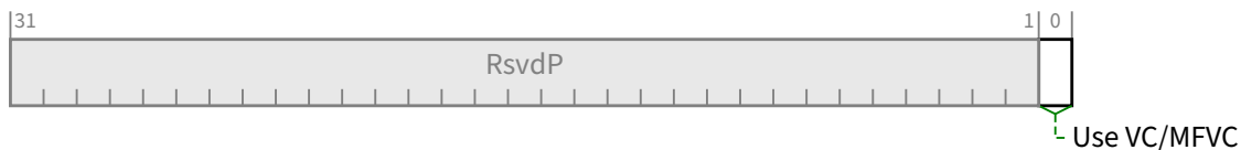
Figure 7-390 SVC Port Status Register §
