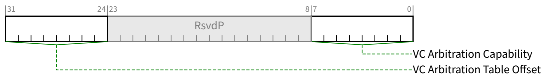
Figure 7-224 Port VC Capability Register 2 §
